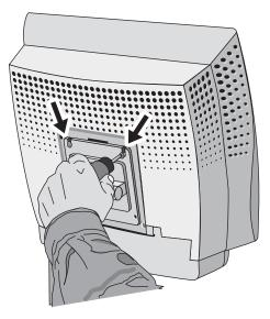
4 Insert and tighten the bottom two screws through the mounting plate.
